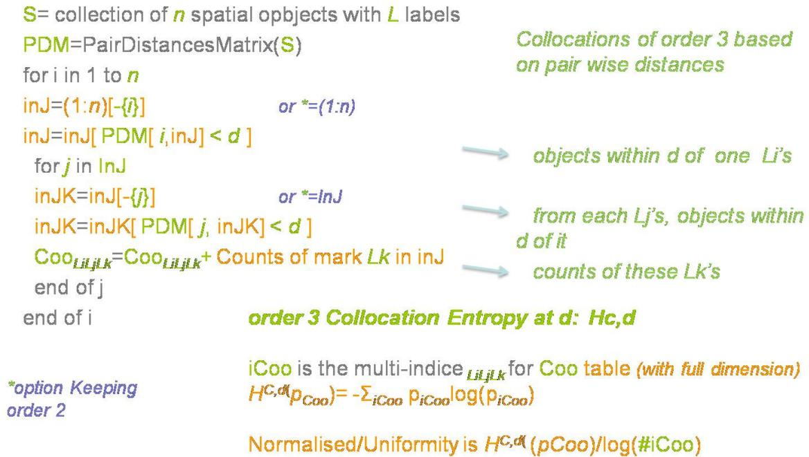
**Figure 1.** Spatial Collocation Entropy and Algorithm to compute cooccurrences table for collocations of order 3
